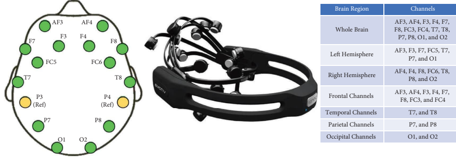
FIGURE 3: Channel locations, Emotiv headset, and channels at different regions of the brain.
